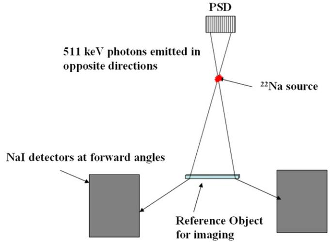
Fig. 3. Principle of Compton scattering imaging technique.
