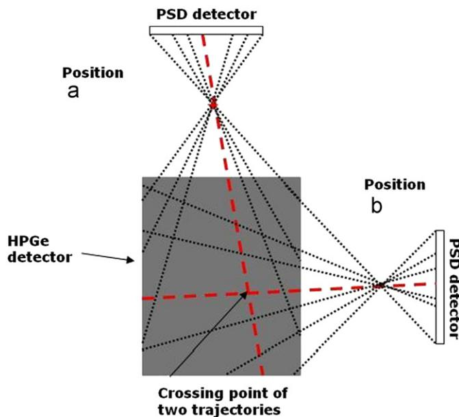
**Fig. 1.** Pulse shape comparison scan of germanium: (a) pulse shapes recorded for the collimation lines coming inside the coincidence cone of PSD and germanium and (b) source and PSD moved together by an angle of  $90^\circ$  and again a data set of pulse shapes is measured.
