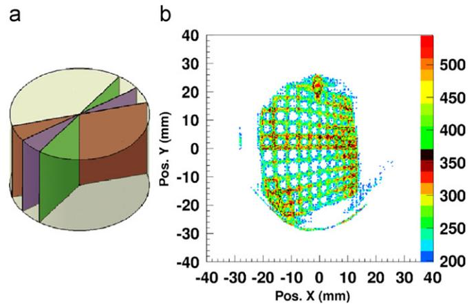
**Fig. 5.** (a) Multiple planes inside the detector volume. (b) Image of the grid when it is rotated by  $40^\circ$ , obtained with the position sensitive detector using the pattern fit algorithm.
