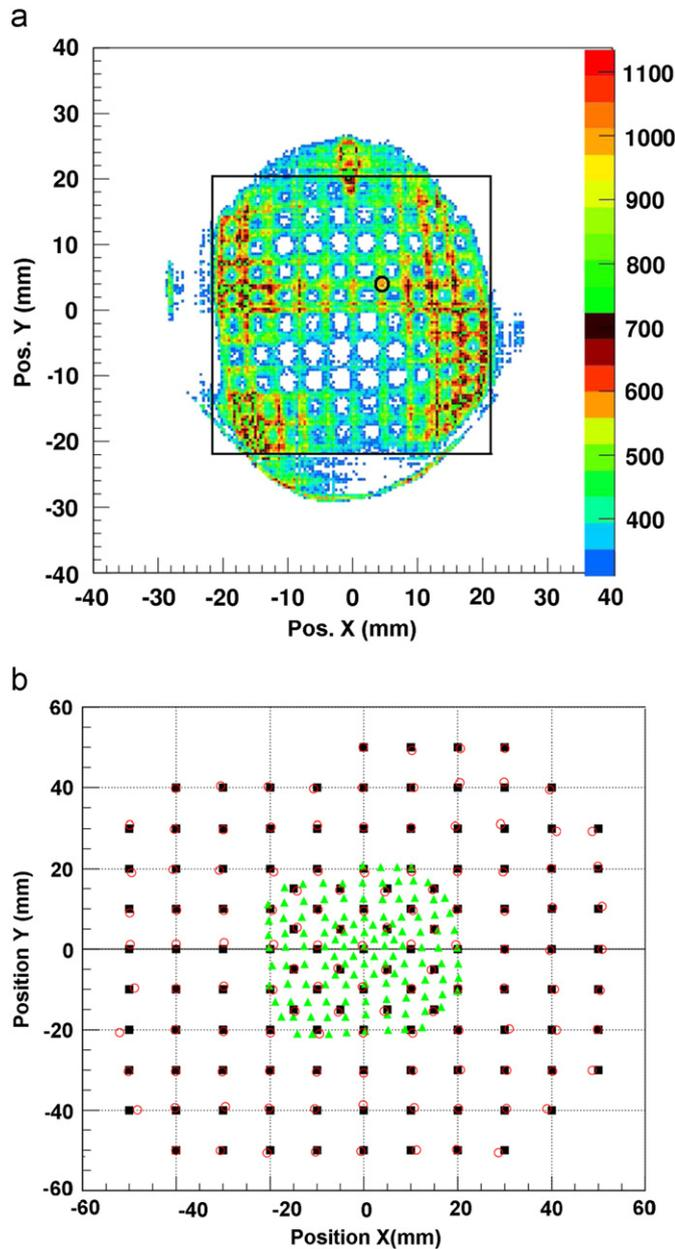
**Fig. 4.** (a) Image of the grid obtained with the position sensitive detector using the pattern fit algorithm. (b) Reconstruction of measured positions by applying 2D functions. The green triangles are the measured positions, black squares are the real positions and the red circles are the corresponding reconstructed points. (For interpretation of the references to color in this figure legend, the reader is referred to the web version of this article.)
