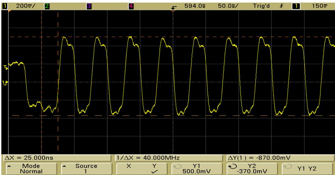
**Figure 9.** First channels of a calibration analogue readout of Beetle 1 corresponding to 51250 e<sup>-</sup>. The first channel is negative, the second positive and so on (25 ns per channel).
