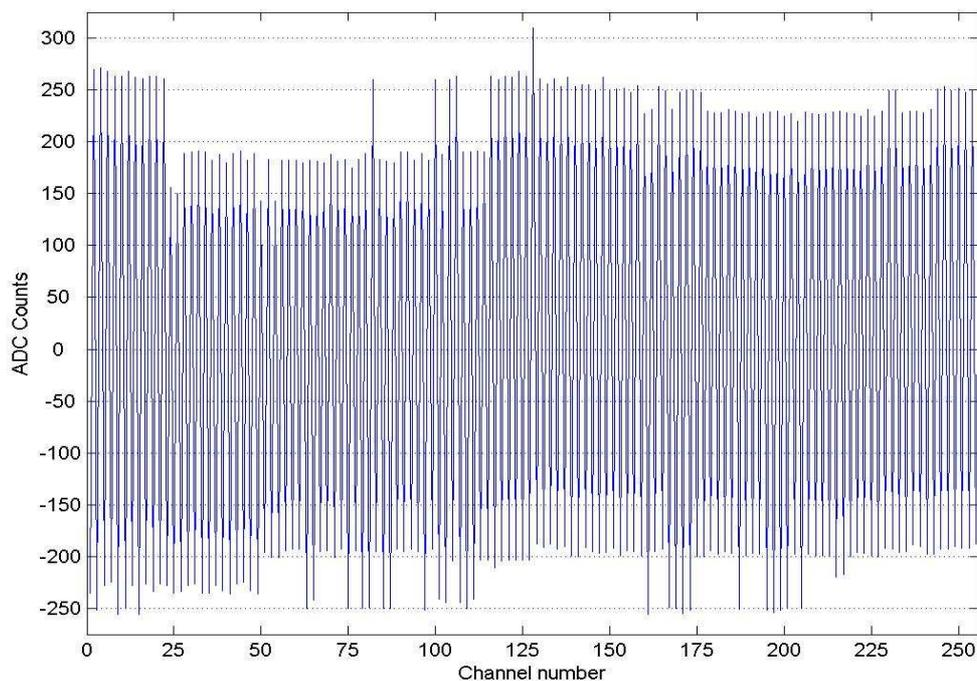
**Figure 7.** Digitized data corresponding to 51250 e<sup>-</sup> with both ADCs operational (channels 1 to 128 correspond to ADC0/Beetle 1 and channels 129 to 256 correspond to ADC1/Beetle 0; 1 ADC count = 2 mV).
