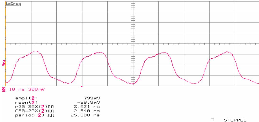
**Figure 5.** Beetle CLK Fast Control Signal (LVDS).
