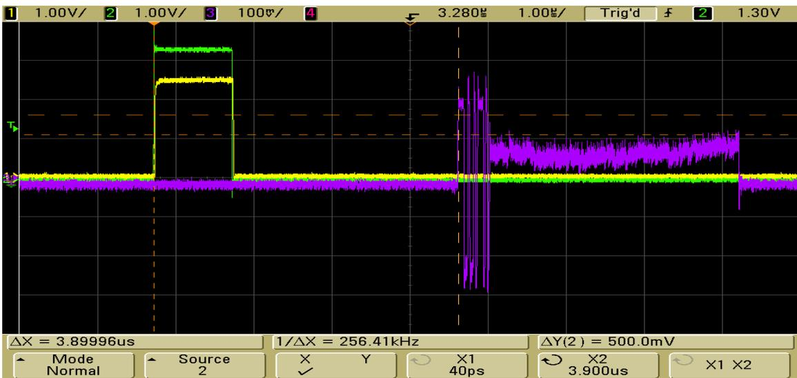
**Figure 15.** Trigger out signal before (green) and after (yellow) being delayed. Analogue readout (purple) for this trigger (no charge). This figure corresponds to a 0 ns delay on trigger out and 500 ns delay on Beetle trigger.
