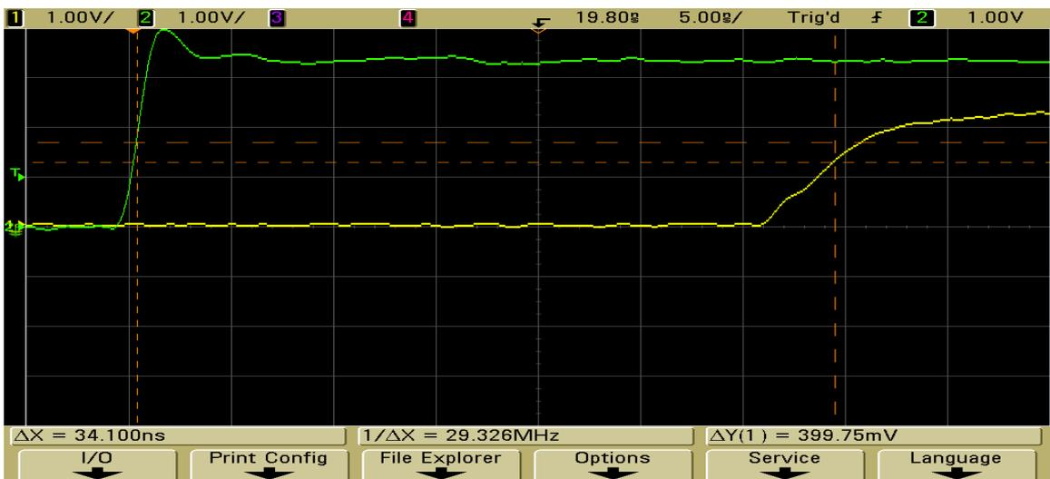
**Figure 13.** Trigger out signal before (green) and after (yellow) being delayed. This figure corresponds to a 20 ns delay on trigger out.
