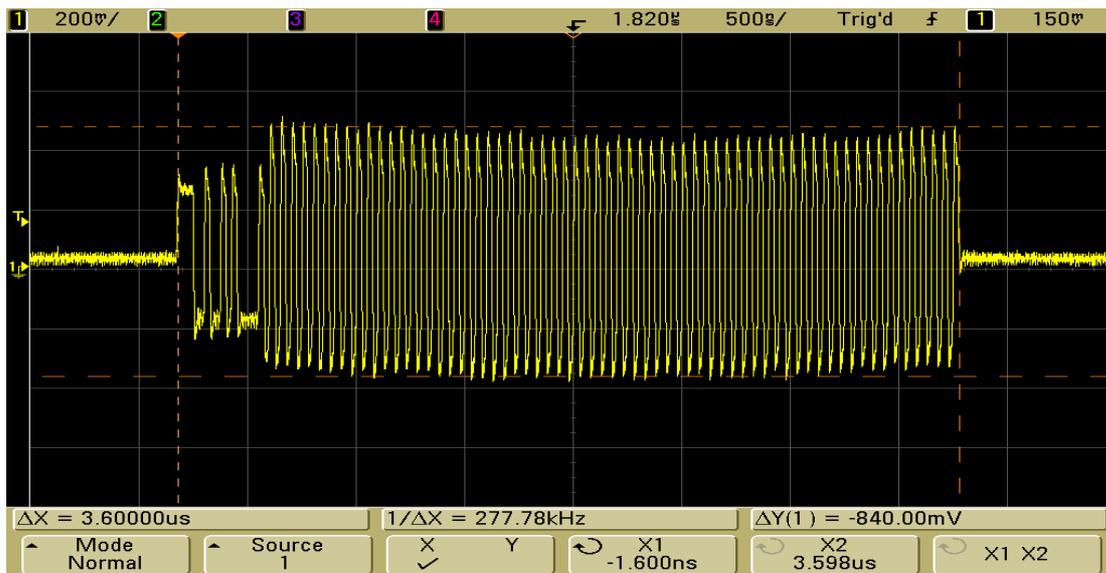
**Figure 6.** Analogue readout of Beetle 0 for a calibration charge corresponding to 51250 e<sup>-</sup>.
