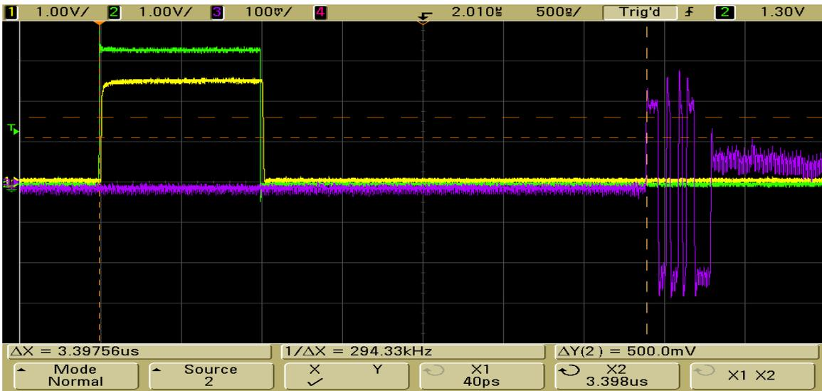
**Figure 14.** Trigger out signal before (green) and after (yellow) being delayed. Analogue readout (purple) for this trigger (no charge). This figure corresponds to a 0 ns delay on trigger out and 0 ns delay on Beetle trigger.
