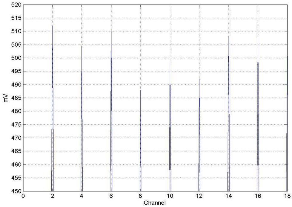
**Figure 10.** First digitized positive channels of a calibration analogue readout of Beetle 1 corresponding to 51250 e-.
