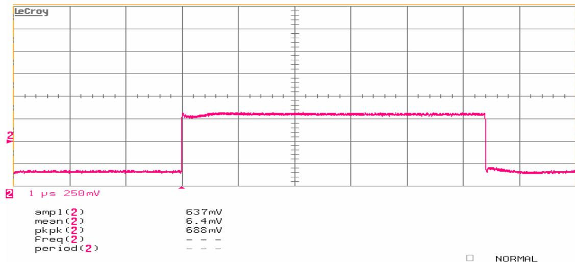
Figure 4. Beetle Reset Fast Control Signal (LVDS).
