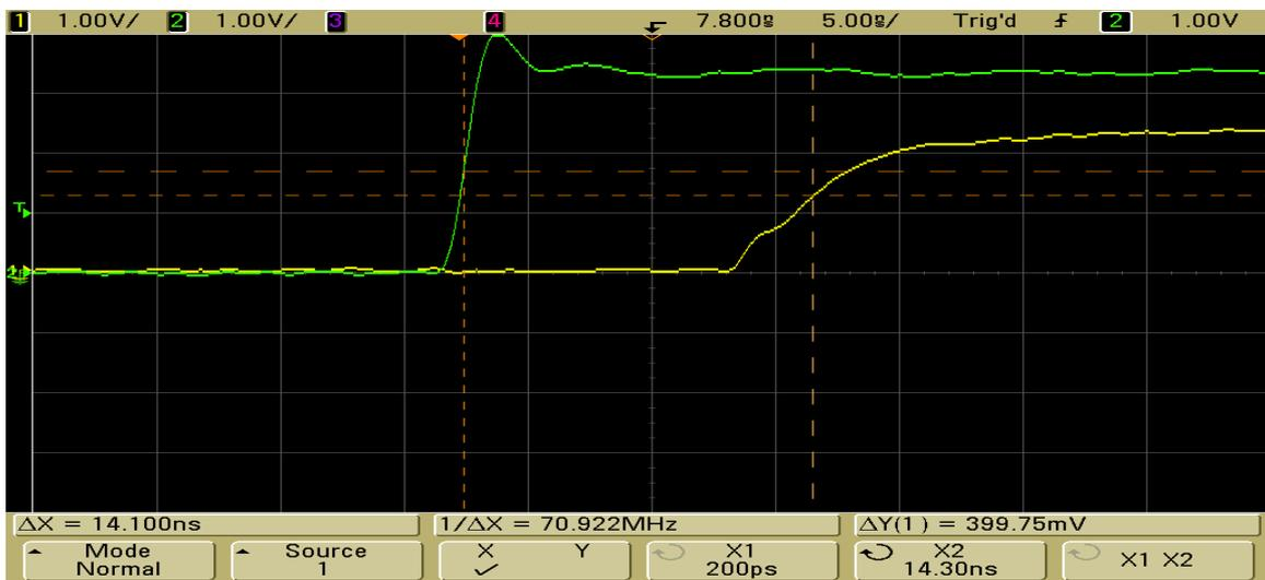
**Figure 12.** Trigger out signal before (green) and after (yellow) being delayed. This figure corresponds to a 0 ns delay on trigger out.
