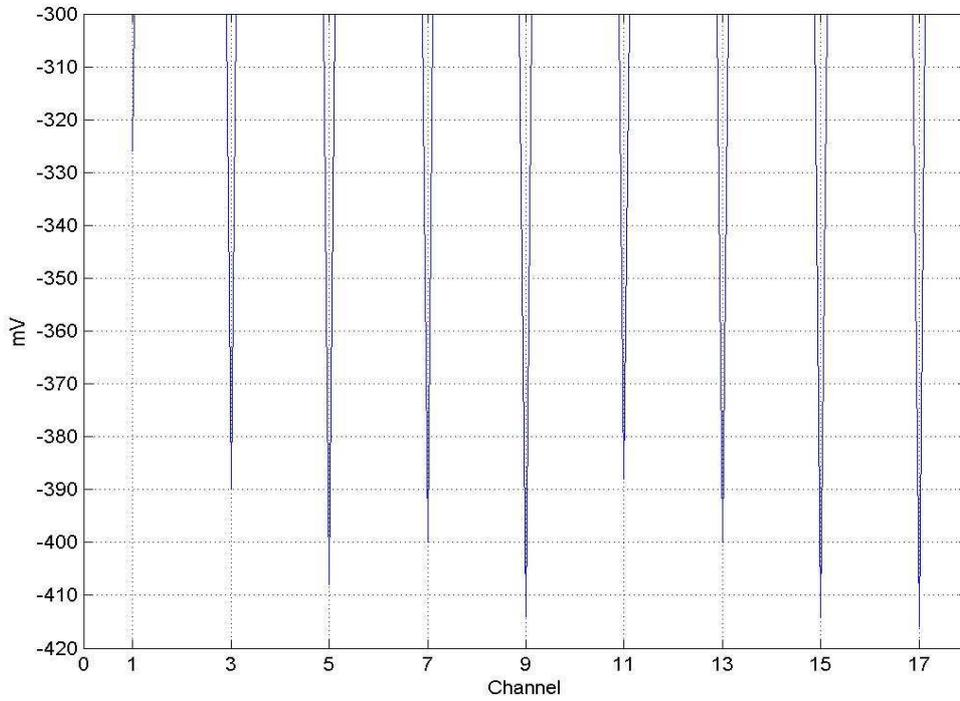
**Figure 11.** First digitized positive channels of a calibration analogue readout of Beetle 1 corresponding to 51250 e-.
