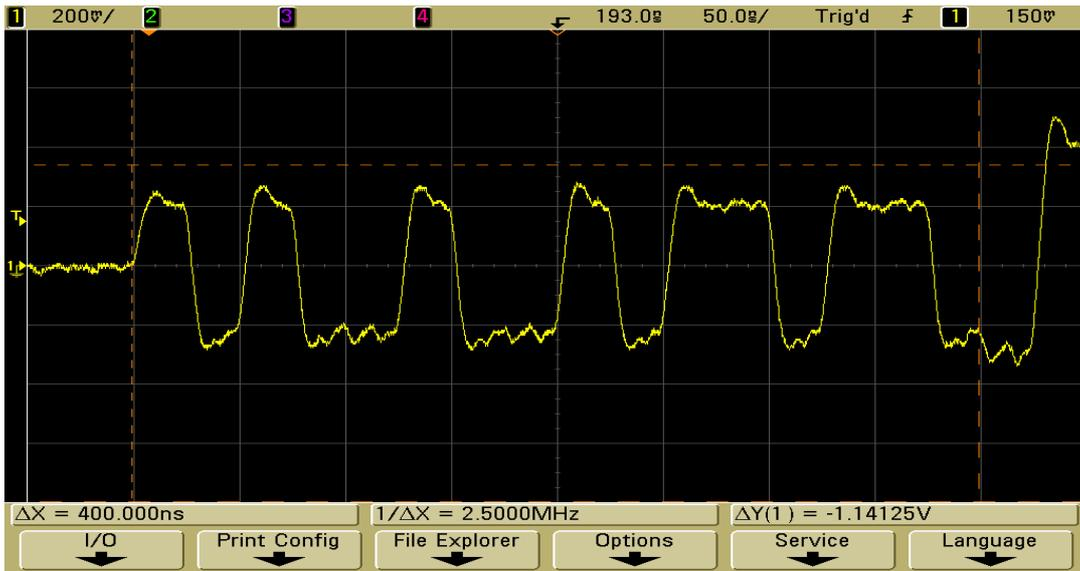
**Figure 8.** Header of an analogue readout of Beetle 1. Header of 16 bits corresponds to 400 ns (25 ns per bit).
