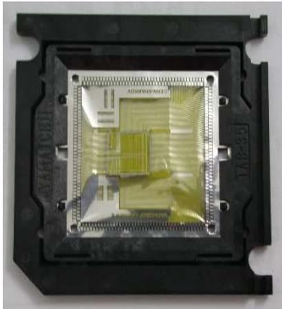
Figure 1. Tabbed chip in the testing frame.
