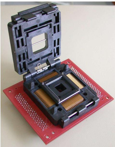
Figure 3. Device to hold the frame with the tabbed chip
