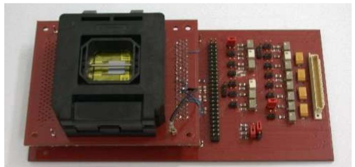
Figure 4. The chip frame and the clamp board are connected to a board that will distribute the DAQ signals.
